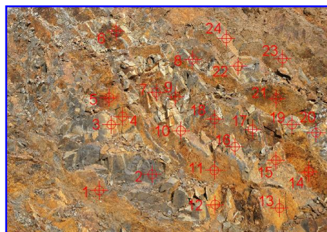
Figure 5: Position of comprasion fractures between photogrammetry method and traditional compass at station 2km+060
