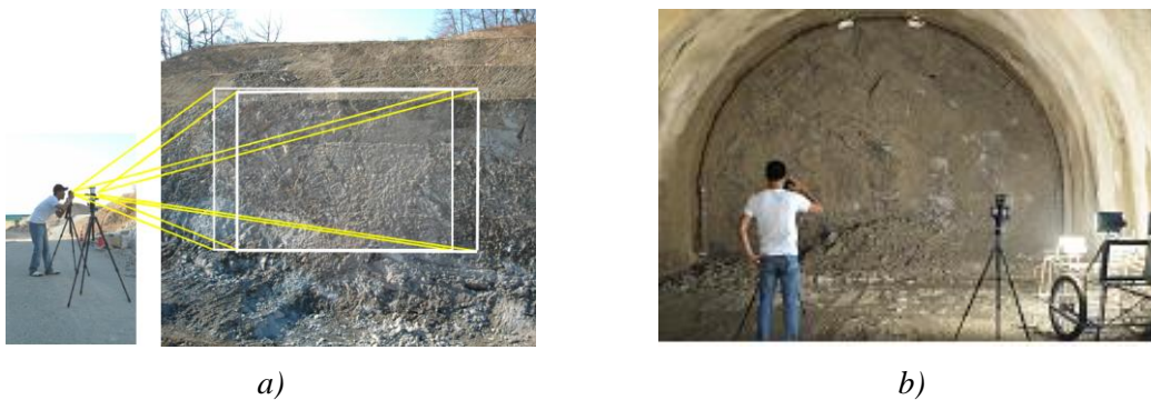
Figure 1. Stereo-pair pictures taken on a slope (a) and inside a tunnel (b).
